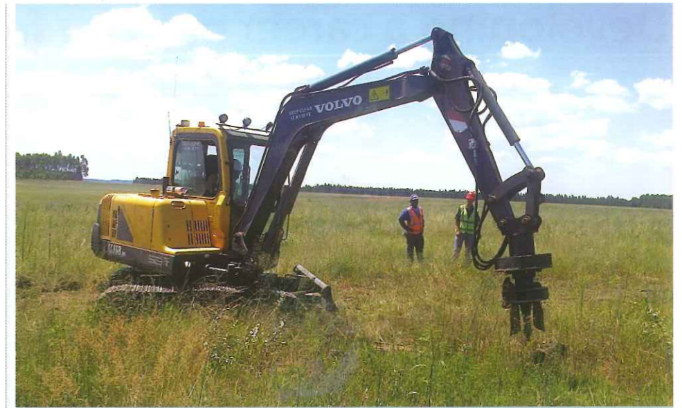
The introduction of new silviculture equipment, like this pitting machine, has provided training service providers with new challenges.
